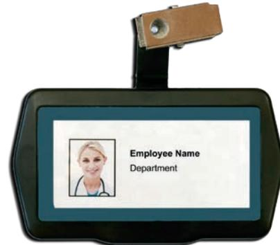
Two-button ID tags provide staff access to offices and patient rooms, as needed, with the press of a button. Otherwise, the tags operate in a handsfree manner. The ID tags additionally include a staff duress feature that enables responders to know the exact location of the staff member in duress and provide a quicker response to the emergency call.
